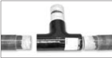
Fig. 7-1. Tapered pipe ready for dry fit.
